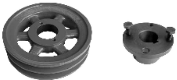
Double Groove "H" Series Cast Iron Bushed Sheave For "4L" & "5L", "A" & "B" Groove V-Belts
