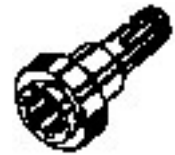
Spring Loaded Collar Rotates About 30 Degrees
